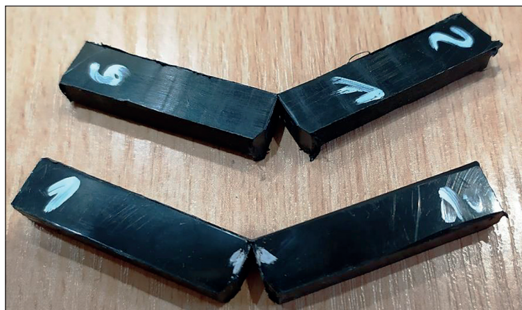
Fig. 4. Exemplary samples after Charpy impact strength test.
