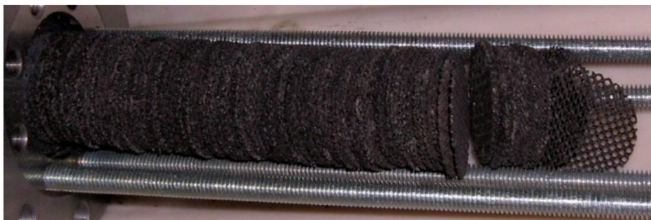
Fig. 3. Wire mesh catalyst, manufactured by Catator [Authors, 2013]
