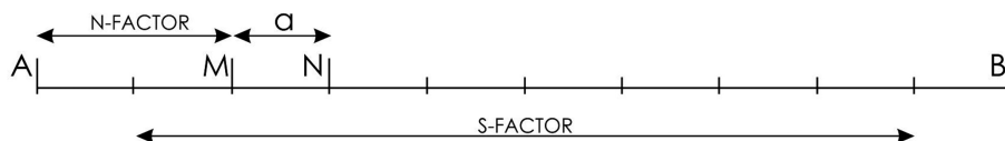
Fig. 5. Sketch of the gradient system showing the position of the electrodes during measurements with the coefficient S = 8 and N = 2 ([36] – modified). AB – supplying electrodes, MN – potential electrodes receiving the current from the medium
