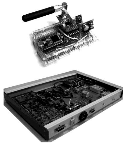
Fig. 11. Universal "remote control" – RollJam (on the left) [11]. Hardware platform for the false GPS transmitter (on the right) [15]
