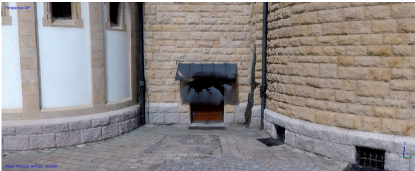
Fig. 9. Distortion of the 3D model: faulty modelling of the door's fragment
