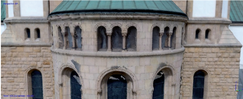
Fig. 8. Distortion of the 3D model: faulty modelling of niche windows
