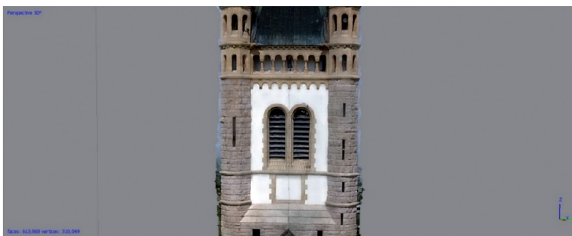
Fig. 11. Distortion of the 3D model: “envelope” around the tower
