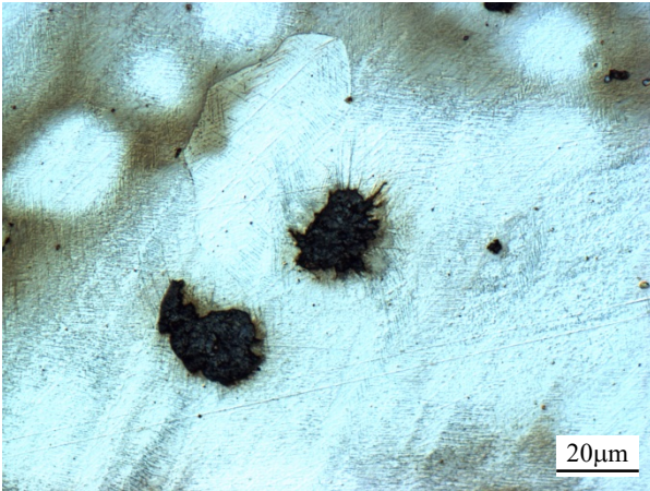
Fig. 8. The representative microstructure of the CGI containing 21.04% Ni in casting with the wall thickness of 24 mm: compacted graphite, austenite
