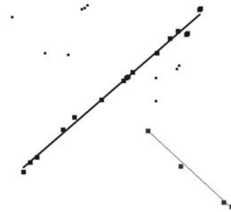
Fig. 4. An illustration of the RANSAC algorithm. The thick line is the best fitted one. The thin line represents a worse line model. The thick line is not biased by the points that were not fitted in the line model.
