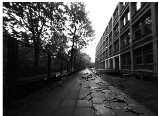
Fig 2. Corners pairing between two successive images. Some corners are mismatched, though as long as these errors are not strongly correlated, the motion is estimated correctly.
