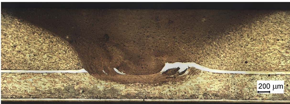
Fig. 3. Macrostructure of FSW aluminum joint
