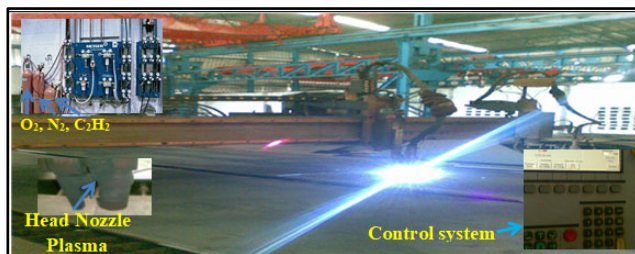
Fig. 1. CNC Plasma Cutting Machine, India/Anand at Gujarat "Elecon Engineering Company Limited"[14]
