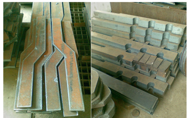
Fig. 2. The cut samples (6) after plasma cutting mild steel with varying the cutting speed and the plasma gas pressure, "Elecon Engineering Company Limited"[13]
