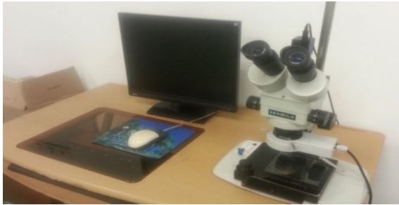
Fig. 4. Optical microscopy to inspection onto kerf width (mag. 1.2x)
