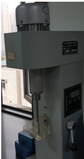
Fig. 2. XFG flotation machine for single mineral flotation tests
