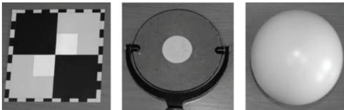
Fig. 3. Targets: (a) b&w, (b) HDS, (c) Faro sphere
