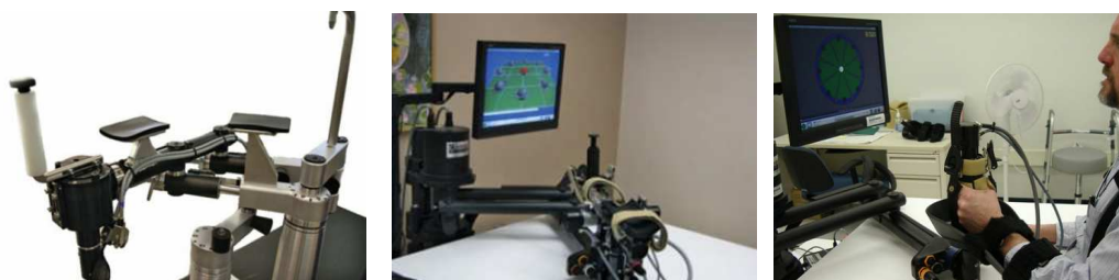
Rys.1. Therapy Robot MIT-Manus [4,7]
