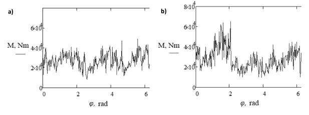
Fig. 1 Changing of the rotational torque which is formed on the head under one turn of the cutting unit in the side cutting mode: if there are all the cutting tools (a) and if there is no 6<sup>th</sup> cutting tool (b)
