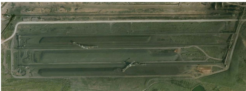
Fig. 7. Three homogenization coal stock of Severočeské doly a.s. – Tušimice on the ortophoto
