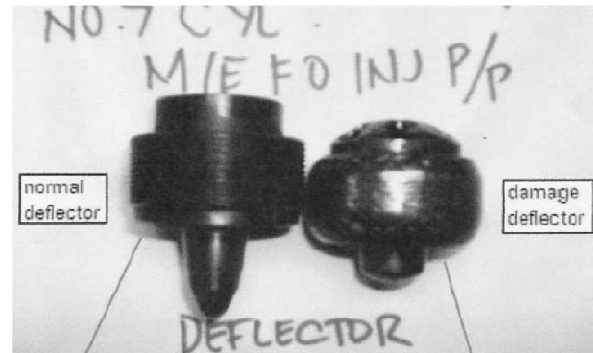
Fig. 11. The example of FIP new and damaged deflector [13]
