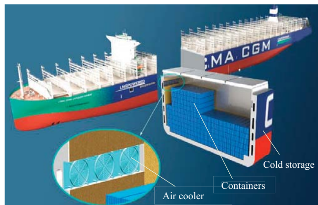
Fig. 3. Model diagram of the new cold storage
