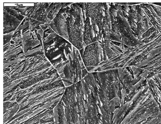
Fig. 1. The microstructure of the steel Hardox-400, 5000x
