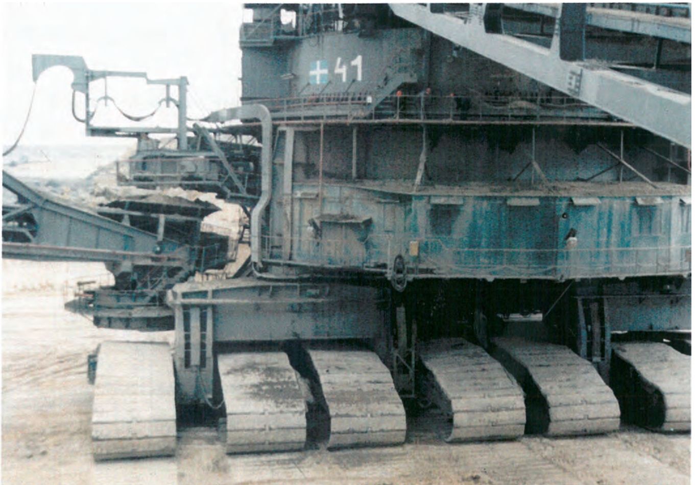
Fig. 1. View of BWE crawler chassis [18]
