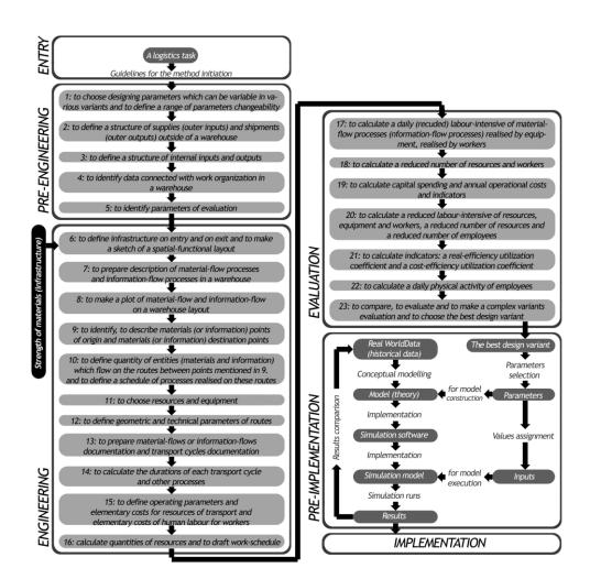
Fig. 1 Scheme of unified warehouse designing method
