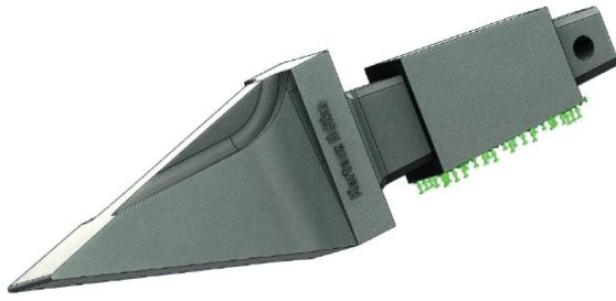
Fig. 8. Fixation conditions of cutting tooth
