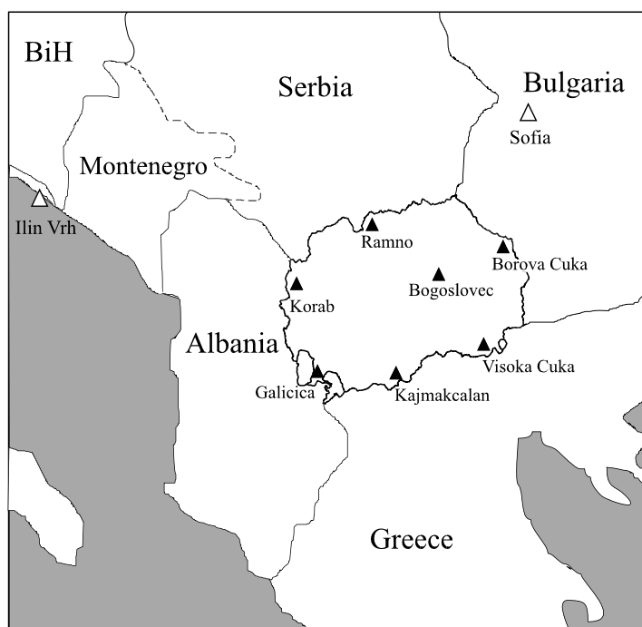
Fig. 4.6.2.1. Points on the territory of R. Macedonia used for merging with the International Reference ITRF 94 Network
