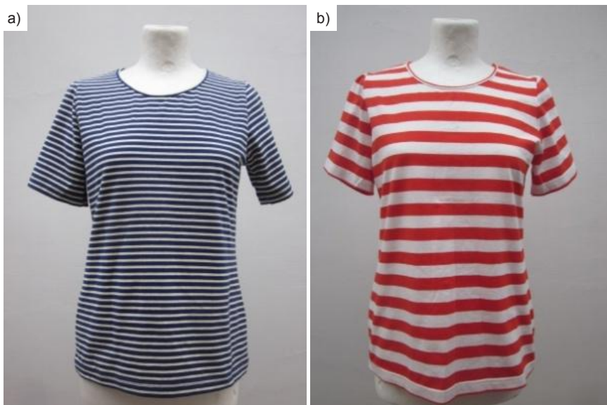
Figure 2. a) T-shirt with narrow stripes: width of stripes 6 mm, repeat of the fabric 12 mm and b) a T-shirt with wide stripes: width of stripes 20 mm, repeat of the fabric 40 mm.
