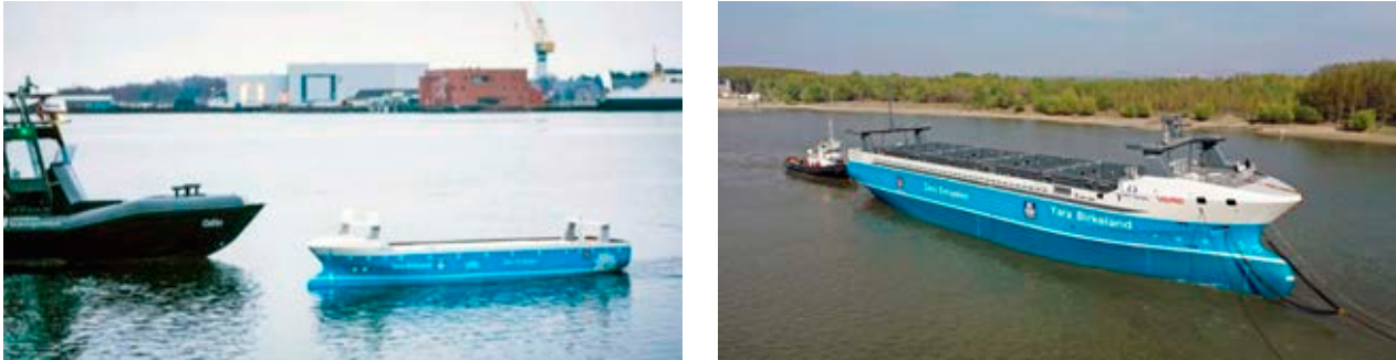
Figure 5. The model of the vessel “Yara Birkeland” for research and testing and autonomous container ship built in 2020 (120 TEU, L = 79.5 m, B = 14.8 m) (GospodarkaMorska.pl, 2020)
