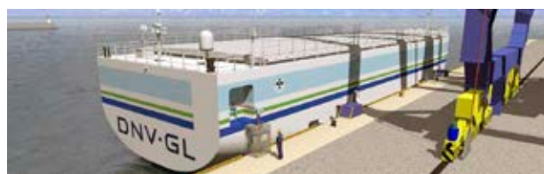
Figure 4. Visualization of the experimental vessel Re-Volt ( L = 60 m; B = 14.5 m; T = 5.0 m; V = 6 knots, range 100 Mm) (DNV GL, 2019)
