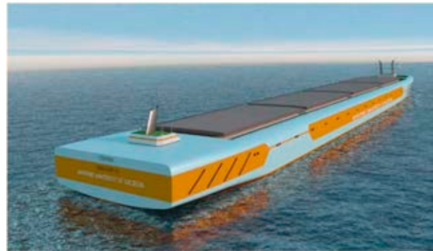
Figure 6. Visualization of the design of an unmanned, autonomously controlled container vessel ( L_c = 78.75 m, B = 11.10 m, T = 4.33 m, \nabla = 2500 m 3 )
