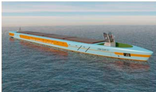
Figure 6. Visualization of the design of an unmanned, autonomously controlled container vessel ( L_c = 78.75 m, B = 11.10 m, T = 4.33 m, \nabla = 2500 m 3 )
