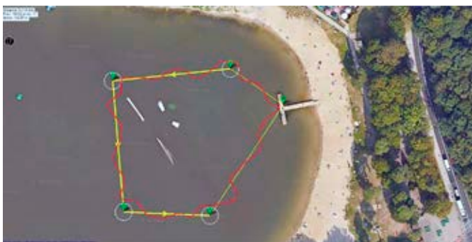
Figure 9. The set and actual route of movement of the model (a) and an exemplary recording of parameters during tests (b)
