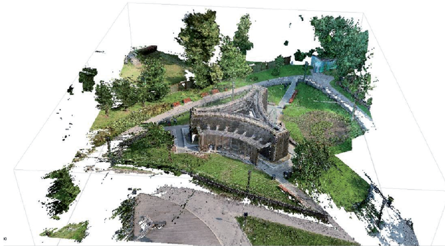
Fig. 7. Dense point cloud generated in Agisoft Metashape
