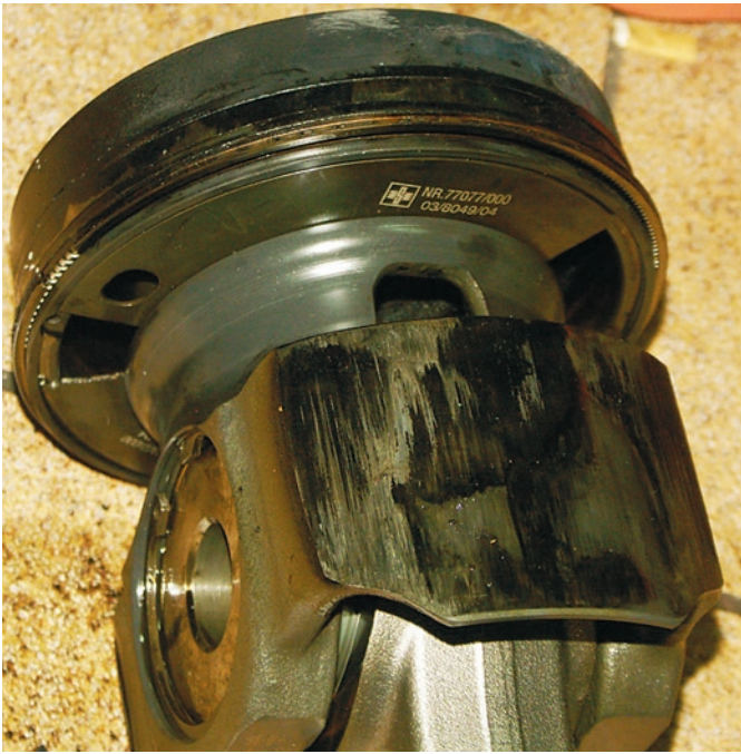
Fig. 5. Piston of dual fuel Caterpillar 3516A engine seized due to failure of oil cooling system of piston crown (photo of the author)
