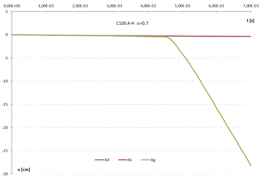
Fig. 7 6a . Change over time of vertical displacements of points in the central section for load level \alpha = 0.7 — detail fig. 7 6 (with a reduced time interval of the analysis)
