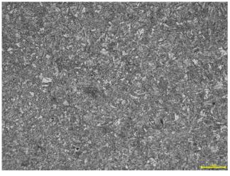
Figure 2 Microstructure of a MAG welded DOCOL 1400M steel weld made using shielding gas (82% Ar + 18%  $CO_2$ ) at preheating temperature of 80°C and welding velocity of 300 mm/min
