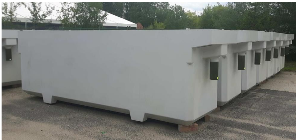
Fig. 1. Newly fabricated electroplating vats
