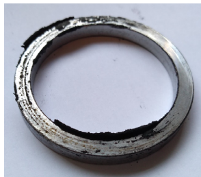
Fig. 5. Steel ring sample after wear test
