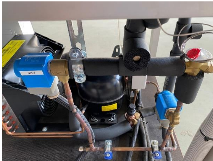
Picture 2. Expansion valves subjected to tests of refrigerant overheating stability
