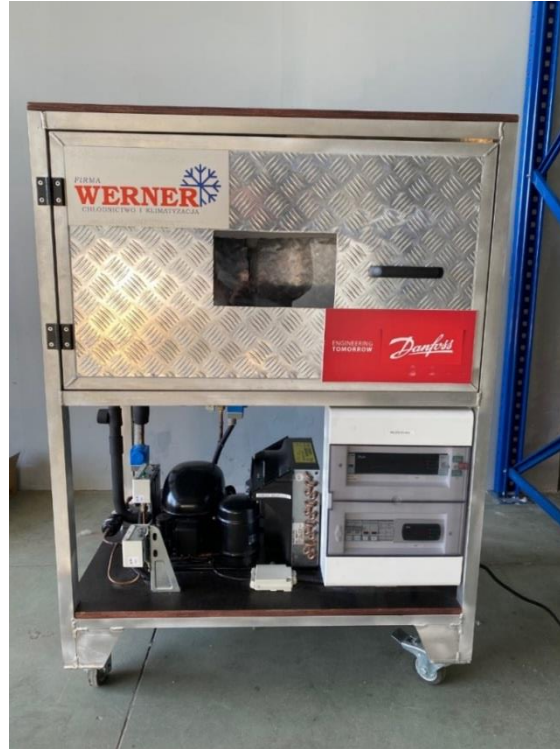
Picture 1. Research stand for refrigerant overheating stability
