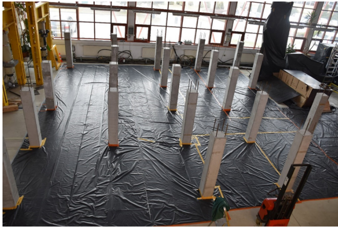
Fig. 2. Prefabricated reinforced concrete columns attached to the strength floor. Source: author
