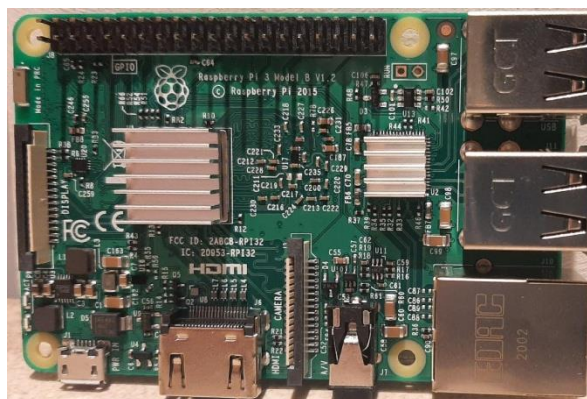
Fig. 2. The Raspberry PI computer with radiators mounted
