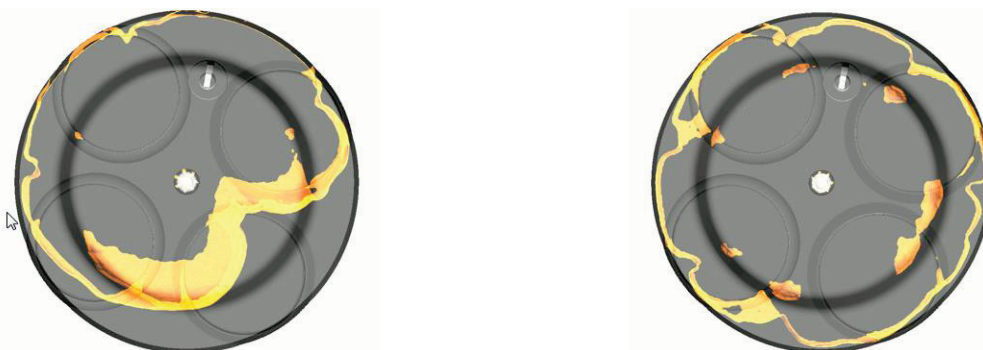
Fig. 3. Open chamber gas engine combustion; flame front position at 5 deg. CA after TDC (left) and 25 deg. CA after TDC (right)
