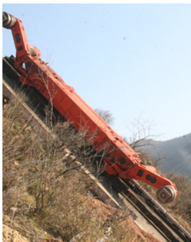
Fig. 5 Classic longwall shearer for strongly inclined seams at the testing grounds of Beijing HOT Mining Tech
