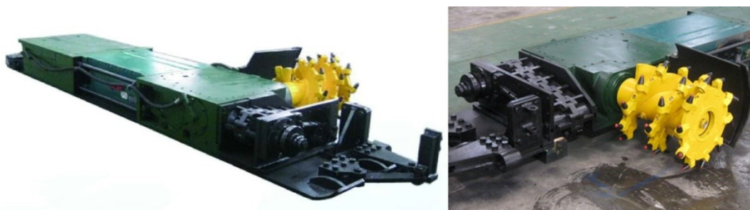
Fig. 3 The HMG100-TP longwall shearer by Mackina-Westfalia S.A. for ultra-thin deposits
