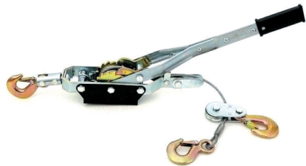
Fig. 3. A winch with a ratchet mechanism [6]
