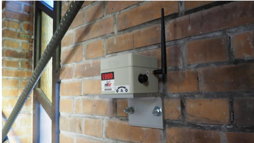
Fig. 6 Biaxial tilt sensor - visible mounting method using a steel bracket anchored to the wall of the structure
