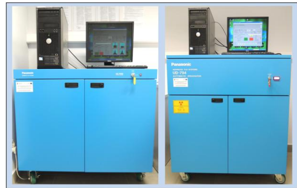
Fig. 3. Reader UD-7900M by Panasonic and Irradiator UD-794
