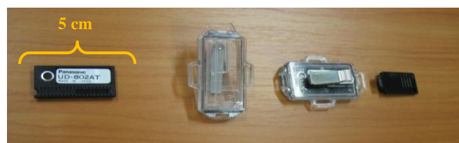
Fig. 2. From the left: UD-802 dosimeter in a protective housing, the case UD-874ATM, dosimeter in a case and the key to open the case
