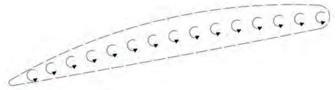
Fig. 1. Modelling a foil with a lifting surface
