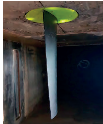
Fig. 7. Foil inside the tunnel – Location 2.
