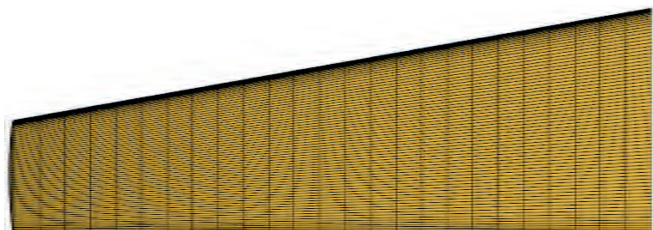
Fig. 10. Computational mesh for RANS-CFD: solid domain
