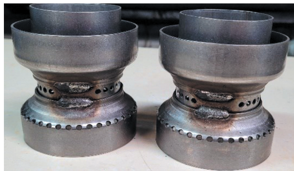
Fig. 1. Exhaust system parts made at the Welding Station AS-03
