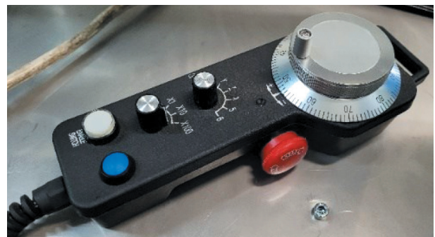
Fig. 6. MPG remote control used for development of the G-code
