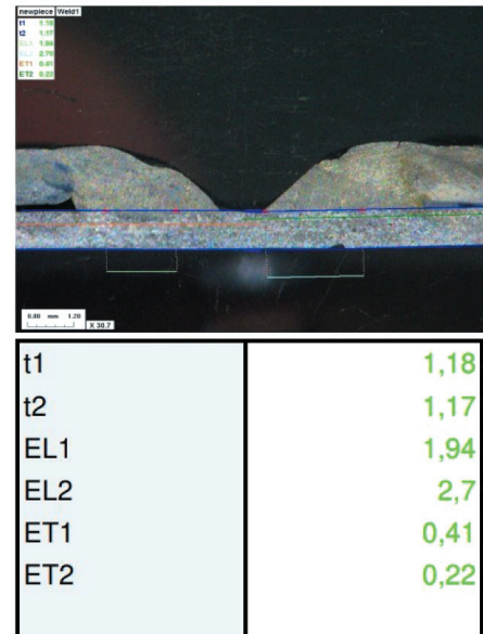
Fig. 8. Part of the metallographic examination report ( t_1 , t_2 – walls thickness; EL_1 , EL_2 – fusion length in the axis of the cut; ET_1 , ET_2 – fusion penetration
