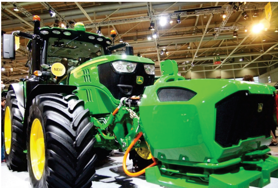
Fig. 3. John Deere tractor with an electricity-generating unit powered by the front WOM as a balance weight
