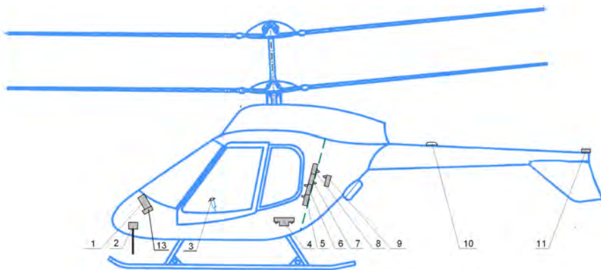
Fig. 6. The layout of the ACS equipment on ULH board
