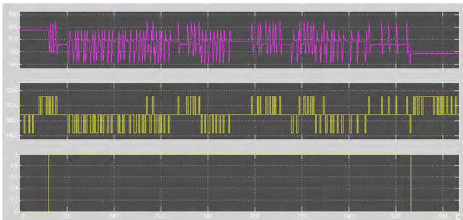
Fig. 8. Work of device of constant RPM ULH „Rotorfly” in time. Control codes from device of constant RPM are shown in the top window. The bottom window shows the level of inclusion of SRS servo of device. The bottom window shows the marks of turning on of the ACS channel
