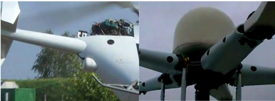
Fig. 2. Installing of parachute recovery system under the tail boom of ULH „Rotorfly” (a) and above the rotor hub of VLH AK1-5 (b)
