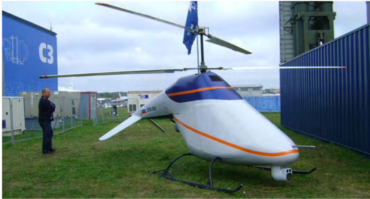
Fig.9. UAV based on two seats ultralight helicopter “Rotorfly”
