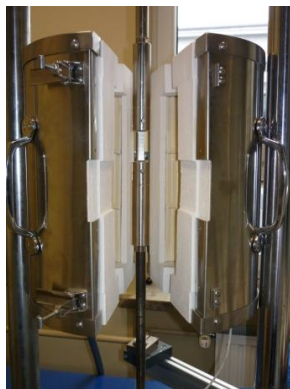
Fig. 4. A view of a specimen for stress-rupture test mounted in retaining holders fixing its position in the creep testing machine furnace heating chamber
