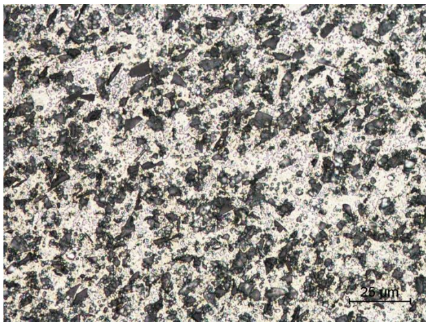
Fig. 1. Microstructure of composite material EN AC-44200 containing 20 vol.% of Al 2 O 3 particles
