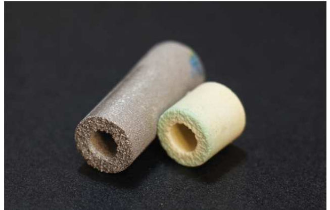
Fig. 4. Metal sleeve (pattern) made in SLS technology and its cast gypsum model
