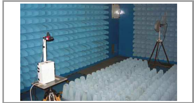
Fig. 4. Experimental set-up. Photograph shows the anechoic chamber used for the experimental assessment of the diplexer prototype.
