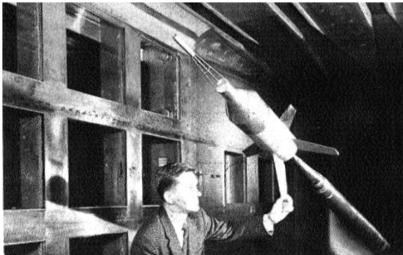
Fig. 7. Tests carried out on a missile model by using the „sting” scales at NASA lab [7]
