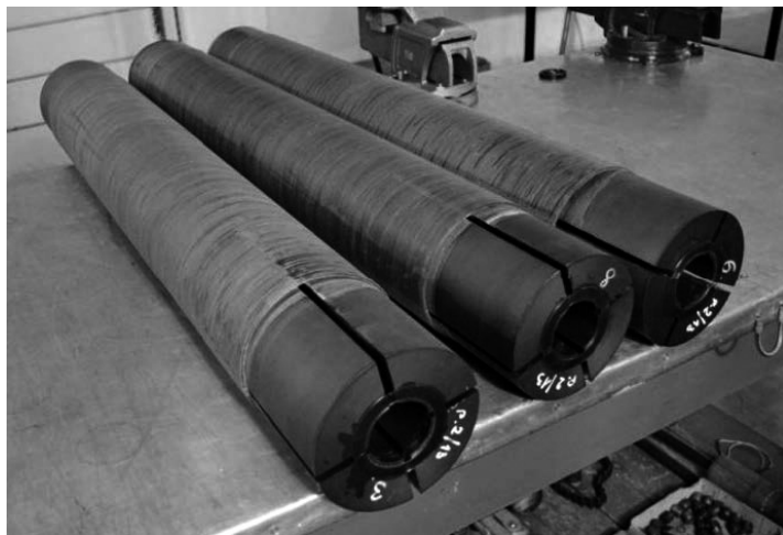
Figure 6. View of a lot of double-base propellant charges for the ballistic tests [14].
