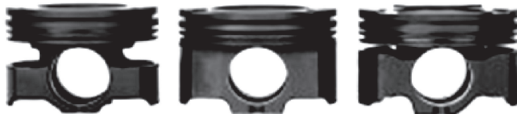
Fig. 7. Steel pistons made by Mahle [24]
