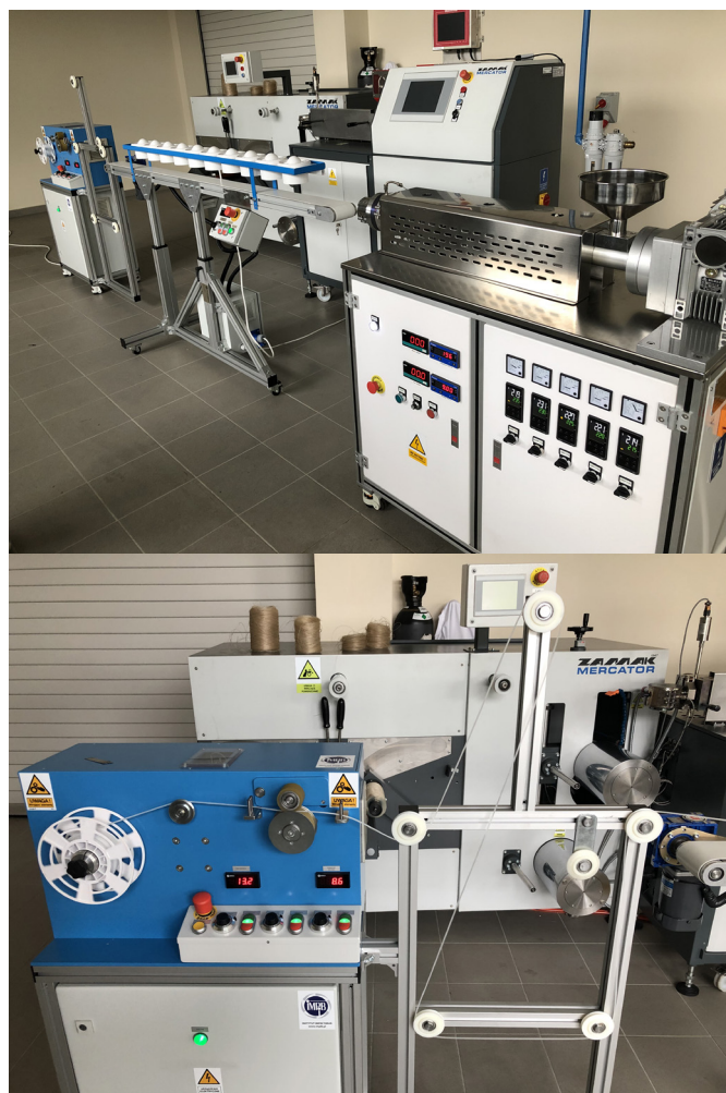
Fig. 2. Original filament production line designed as part of the work
