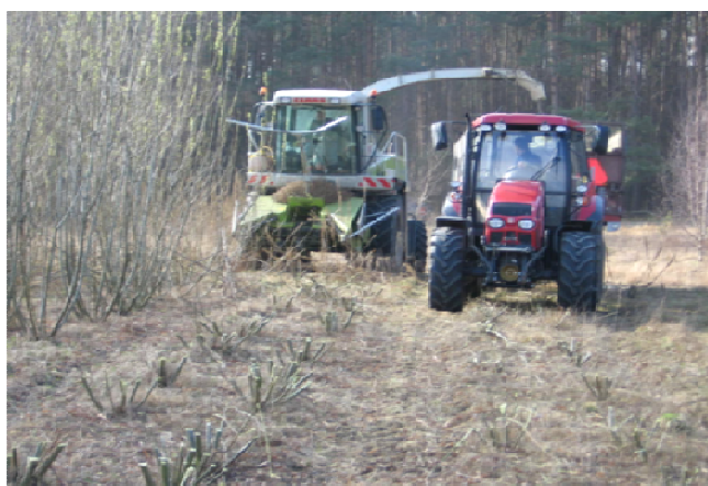
Fig. 2. One-step willow harvest with the use of Claas Jaguar 83 chuff-cuter. Source: Photo from own archives
